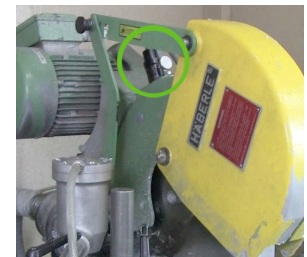
Example of easily mounting a Bat Nozzle to a circular saw.
