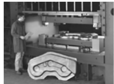
A typical die set application using wear plate L blocks and bosses for stamping of a large, heavy gauge part.
