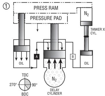
As press ram comes down, oil from prime cylinder is pumped into top side of delay cylinder.
