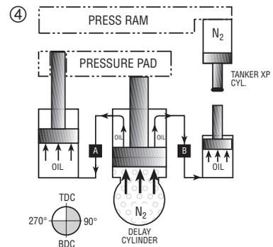
At a customer-determined point in press stroke, valves A & B open, allowing fluid from top side of delay cylinder to return to prime and timing cylinders.
