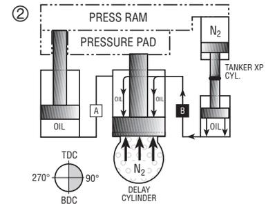
At or near bdc, valve B opens, allowing Tanker XP cylinder to extend, depressing timing cylinder which pumps oil into top side of delay cylinder. This achieves lockdown, zero pressure exerted on pad from delay cylinder.
