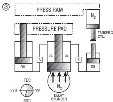
As press ram goes up, delay cylinder and pressure pad remain in lockdown position.
